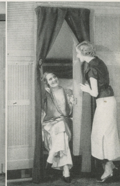
When a section is prepared for single occupancy, the upper berth is not used. A sliding louvre-door, for proper ventilation, makes the section completely private. When the door is closed by occupant of berth the protruding curtain folds down flush with the exterior of the section.
