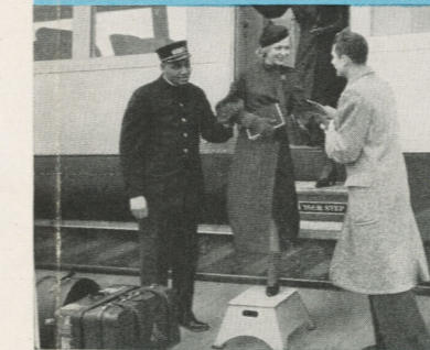
The doors of the new train, when closed, form a part of the smooth exterior of the cars. The doors interlock with the steps which fold up and down as the doors are closed or opened.
