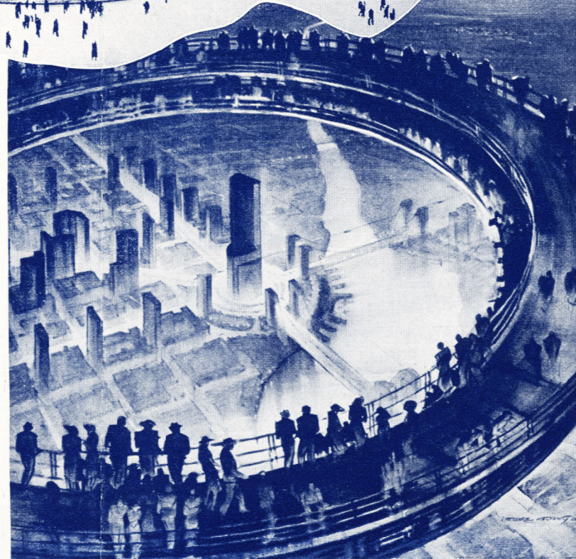
Cut-away drawing shows the Theme Center of the New York World's Fair 1939. This unique twin structure will house the focal exhibit of the Exposition. The drawing shows: 1—Perisphere, a 200-ft. sphere. 2—Trylon, a 700-ft. triangular obelisk. 3—Entrance to exhibit. 4—Escalators carrying visitors to 65-ft. level. 5—Revolving platform from which to view the interior. 6—Model of the City of Tomorrow. 7—Exit Bridge leading to descending ramp. 8—Heliograph or Exit Ramp encircling the structures.
