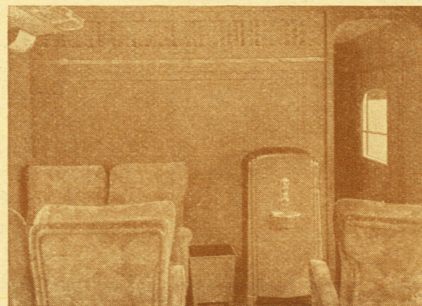
Electric Water Cooler
