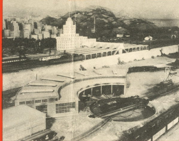
The roundhouse: home of the iron horse; a freight engine on the turntable is headed for its designated track.
