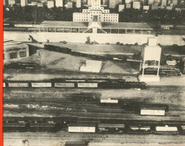
Classification yard; freight cars are classified on different tracks for assembly into trains going to various destinations.
